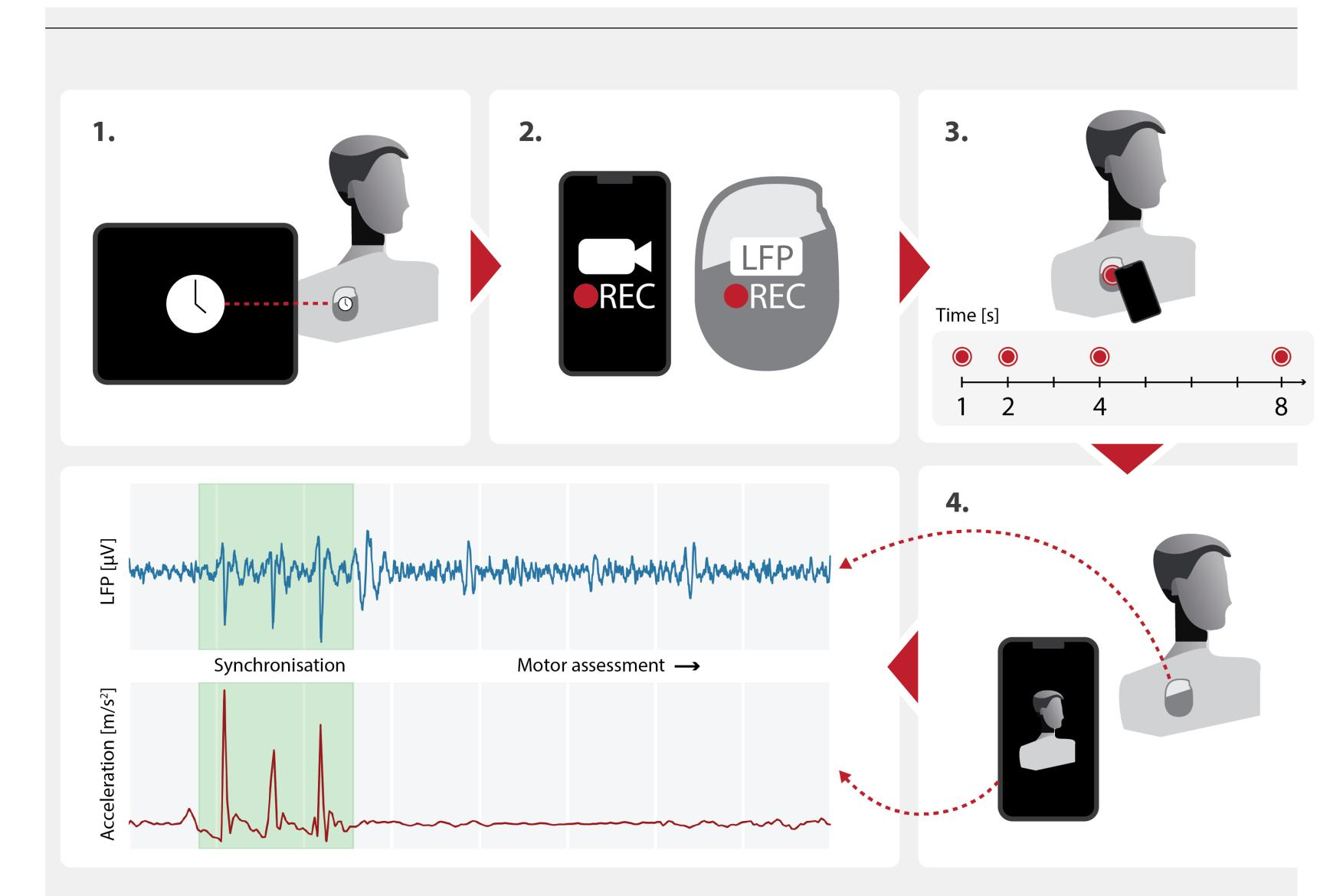
Figure 1. Data capture procedure. After updating the internal clock of the DBS device through its control tablet, the video and LFP capture is initiated. LFP signal artefacts get induced through a series of taps made with the video-recording mobile device. The same device is then used to capture the subsequent motor assessment. The LFP signal gets aligned with the mobile device's accelerometer reading which results in LFP-video synchronisation.
